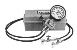
The Dual Hose Meter Kit includes a pressure gauge with dial, three-way push button-operated valve, 5' long dual connection hoses, dual shut-off valves, and carrying case. Choice of fittings for connecting unit to either a pressure valve or pressure / temperature valve.
