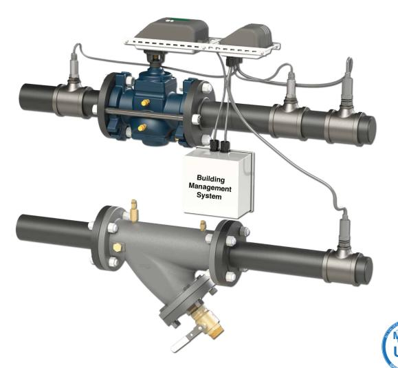
The EPIC System measures energy usage while monitoring coil performance to adjust a Pressure Independent (PI) Control Valve to optimize coil performance. The PI Valve maintains the correct flow, in spite of pressure changes, and guarantees the flow only changes when demand requirements change or Delta T is outside of specification.
