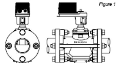
4. All other sizes: 8 holes flanges require (8) 5/8" X 2-3/4" bolts and (4) 5/8" X 12-1/2" studs. 2-1/2" to 4" valves are compatible with both Class 150 and Class 300 flanges. 5" valve is compatible with Class 150 flanges and/or Class 300, 5" flanges
