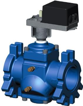
1. Clean the lines upstream of valve particles larger than 1/16" diameter (welding slag, pipe scale and other contaminants). Griswold Controls recommends the use of a strainer upstream to prevent damage or blockage.
