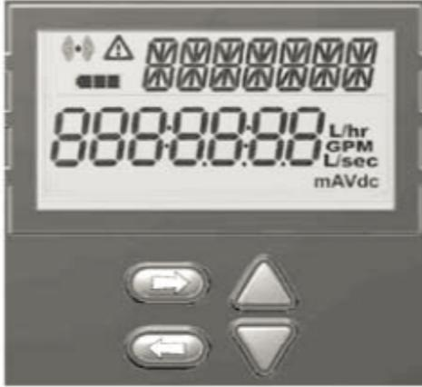
The programming menu is always accessible. To enter the programming menu, please simultaneously press the two arrow buttons (→ and ←) for 6 seconds, until bottom line blinks.
