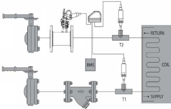
The BTU Meter measures flowrate, Delta T, and calculates energy usage.
