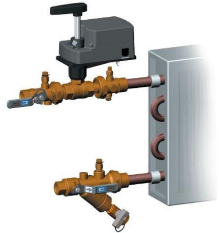
Valves included in standard piping packages are all Next Generation, which contain triple seals and field repairable stems. These Next Generation valves provide resistance to chemical treatments and temperature fluctuations following evening system shutdown, and allow for field servicing without removing the valve.
