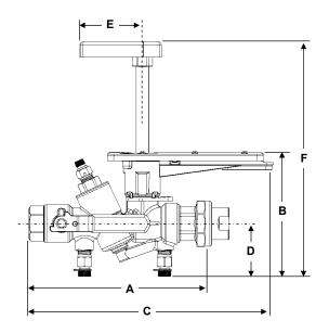
NOTE: The PIC-V is available with fixed x fixed ends or fixed x union ends. (fixed by union shown)
