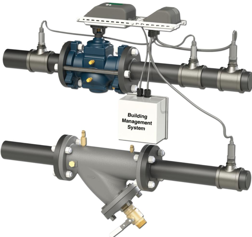
The FIT Energy System measures energy usage while monitoring coil performance to adjust a Pressure Independent (PI) Control Valve to optimize coil performance. The PI Valve maintains the correct flow, in spite of pressure changes, and guarantees the flow only changes when demand requirements change or Delta T is outside of specification.
