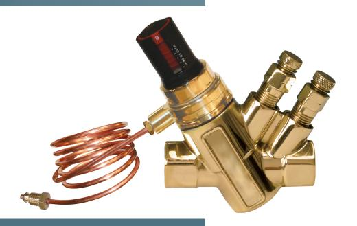
PIM<sup>™</sup>-A Mini controls the differential pressure across a coil, valve, or circuit. By controlling the pressure differential you can maintain design flow regardless of pressure changes. Controlling the differential pressure also reduces the risk of noise from control valves as they close as well as noise in radiators when pressure increases.
