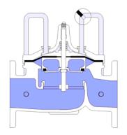
**FULL OPEN OPERATION** When pressure in the cover chamber is relieved to a zone of lower pressure, the line pressure at the valve inlet opens the valve, allowing full flow.
