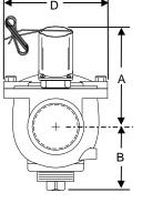
Operating Pressure:3 to 80 PSIMaterial:Cast Iron and BroEnd Connections:NPT (BSPT OptioVoltage Operating Range:22-28 VACLow Current Requirement:0.10 A at 24 VACAssembly:Valve comes fully
